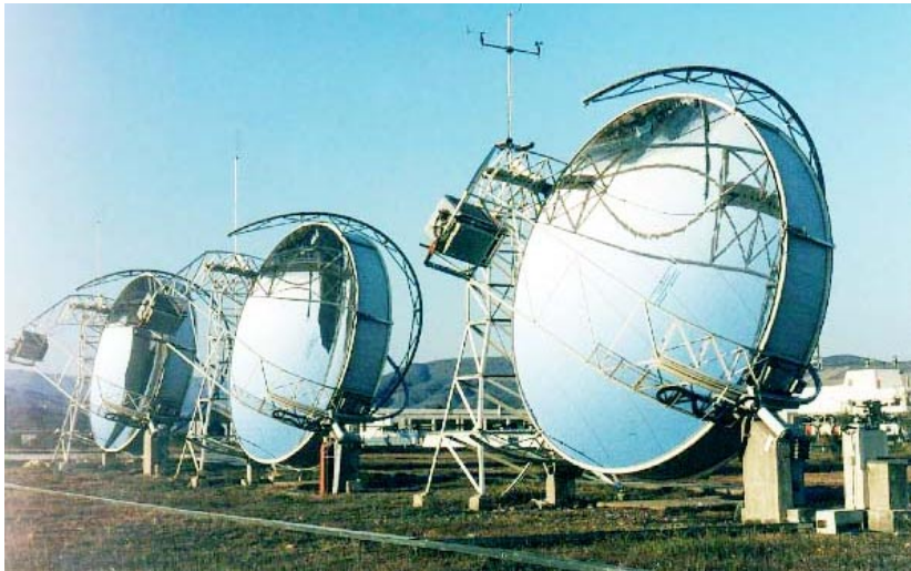
Figure 9: Dish/Stirling System (Schlaich, Bergemann and Partners, engine from SOLO) tested at the PSA
